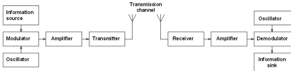
*Figure 7 - Radio Communication System*
