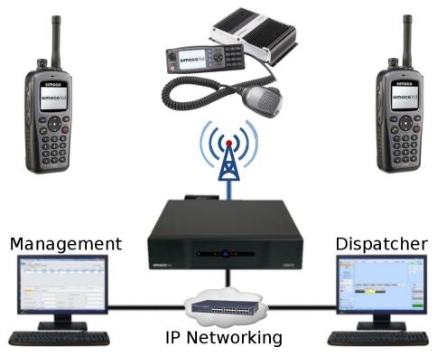
A single base station is usually installed where the coverage area is required to be extended beyond the range that can be achieved with terminals working in direct mode. Provision of a base station also enables the connection of dispatchers, network management and third party applications. Each base station can be configured with a SIP telephony trunk to enable radio to telephone calls.
