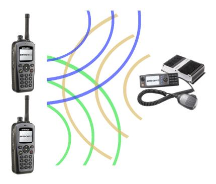
The simplest use of Simoco Xd products is where DMR radios are deployed without any fixed infrastructure and communicate using direct mode operation. Both portable and mobile radio terminals can operate in this mode, either in environments where a small operational area means that coverage can be achieved without a base station repeater or in situations where terminals need to work outside of their normal system coverage area for a period of time.
