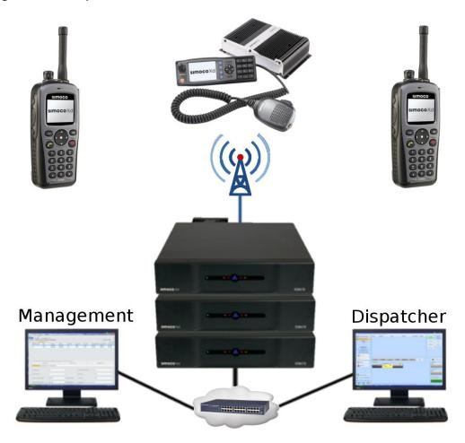
In order to provide additional capacity on a site for larger numbers of users, additional base stations can be installed, each providing an additional two timeslots and requiring its own 12.5kHz frequency pair. Base stations are connected to the antenna through a combiner. An Ethernet switch is installed at the site if there is a requirement for communications between base stations or for the DMT/applications to connect to the base stations over IP.
