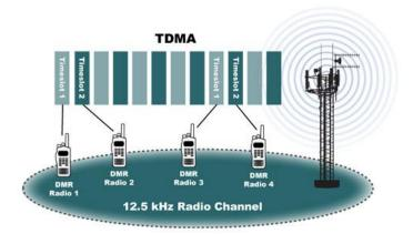
Since the TDMA technology enables the 2 digital timeslots to fit within a standard 12.5kHz analogue channel, this means that Simoco Xd can be deployed within existing analogue frequency spectrum. Users can therefore easily migrate from analogue radio systems to take advantage of Simoco Xd without any re-licensing issues and can benefit from increased capacity and/or reduced license costs immediately.
